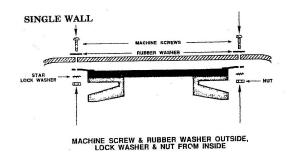
**Note:** On vehicles with single wall or fiberglass, drill the 11/64" holes through the wall or roof. Mount with the machine screws, rubber washers, and nuts provided.
